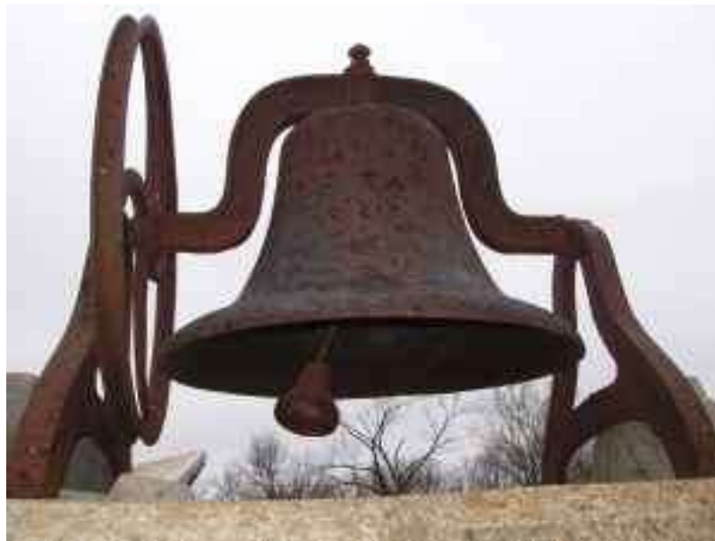
A 1900s Cast Iron Church Bell, complete with bell, yoke, clapper, stand and pulley (pulley wheel) Measures 25 1/2" Diameter, Wheel measures 26" in diameter The Number 26 is on the yoke
